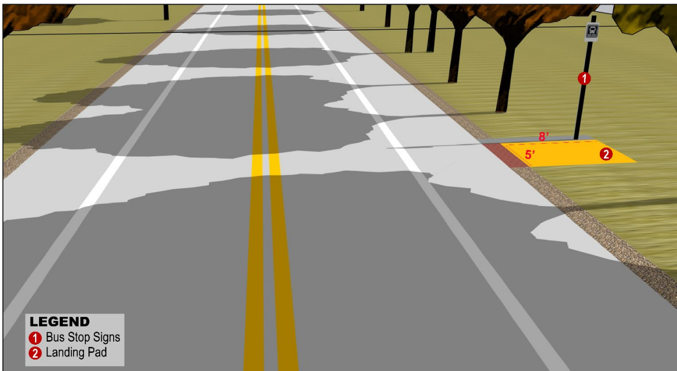
Figure 50: Accessible Bus Stop without Sidewalk Access
